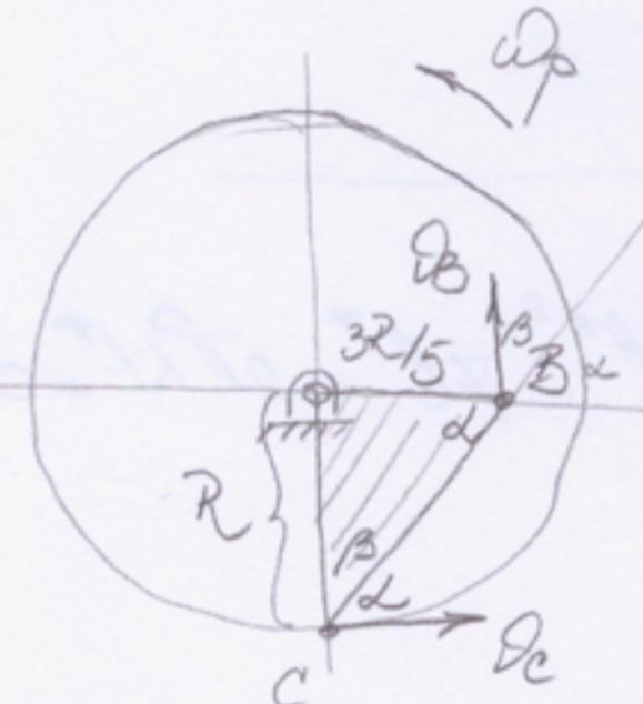
$$\operatorname{tg} \alpha = \frac{R}{3R/5} = \frac{5}{3} \Rightarrow \underline{\underline{\alpha}} = \arctg \frac{5}{3} = \underline{\underline{59,04^\circ}}$$
