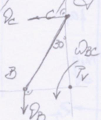
$$\omega_B = \overline{BP} \cdot \omega_{BC} \rightarrow \underline{\omega_{BC}} = \frac{\omega_B}{\overline{BP}} = \frac{\omega_B}{BD} = \frac{2\sqrt{3}}{\frac{\sqrt{3}}{2}} = 4 \text{ rad/s}$$
