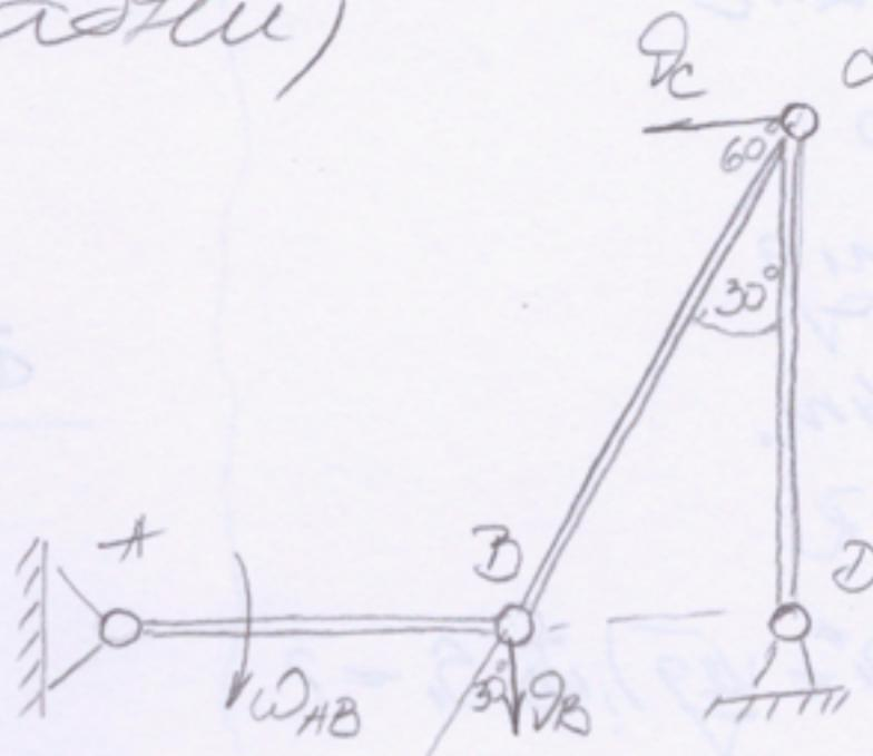
$$\vec{\omega}_B \perp \vec{AB} \quad \vec{\omega}_C \perp \vec{CD} \quad \omega_B = AB \cdot \omega_{AB} = 2\sqrt{3} \text{ rad/s}$$
