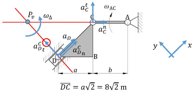
$$a_{c_t} = \overline{AC}\varepsilon_{AC} = 3 \cdot 1 = 3 \text{ m/s}^2, \quad a_{c_n} = \overline{AC}\omega_{AC}^2 = 3 \cdot 2^2 = 12 \text{ m/s}^2$$
