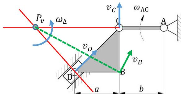
$$\overline{BP_v} = \sqrt{BC^2 + \overline{CP_v}^2} = \sqrt{8^2 + 16^2} = 8\sqrt{1+4} = 8\sqrt{5} \text{ m}$$
